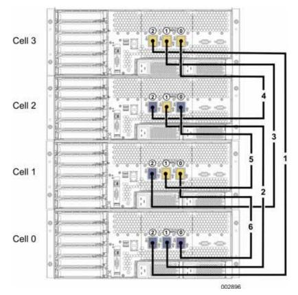
Figure 3-3 System with Four Cells
